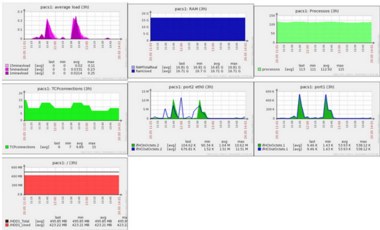
Figure 3. The Zabbix Control Panel Monitoring the PACS Server with SNMP
