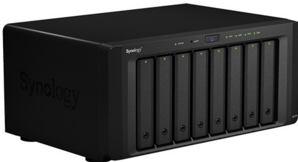
Figure 4. My Synology 1815+ has eight drive bays populated with 6TB drives. The software is amazing, and it includes cloud syncing to Amazon Cloud Drive.
