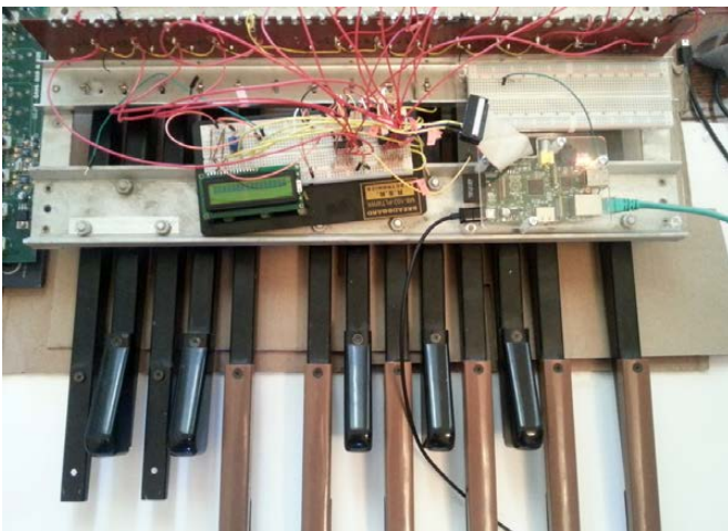
Figure 3. @josephbottinger's RPI runs a midi foot controller AKA Alcyone Beta
