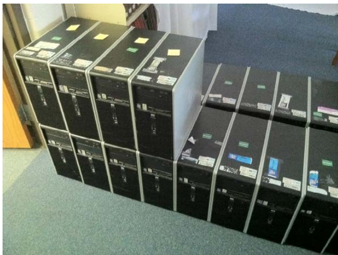
Figure 1. Old workstations make perfect LTSP thin clients. These machines were donated as junk, but they'll make excellent student workstations.
