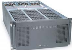
5U-48Bay 96TB Storage Server
