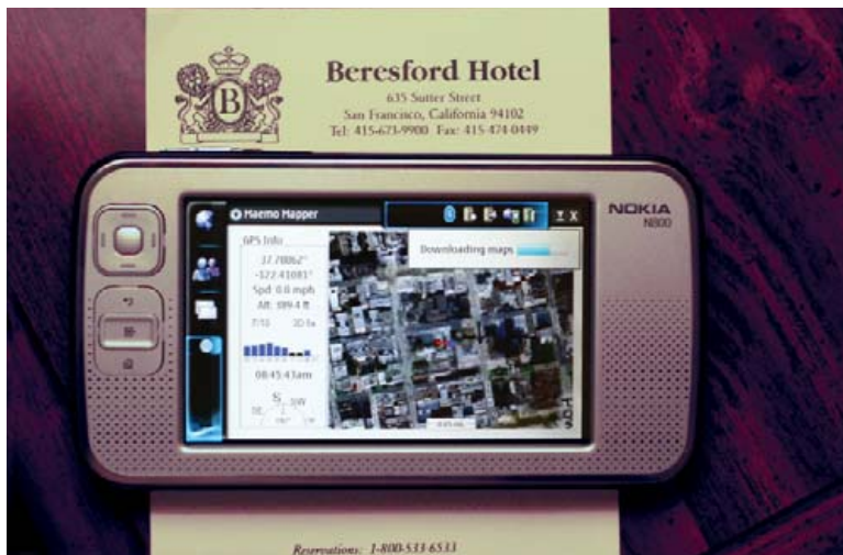
Maemo Mapper at the hotel in San Francisco. The GPS receiver was at the window on one side of the room. The N800 here was on a table across the room near the door. Over on another table was the Nokia E62 mobile phone, which the N800 used for downloading maps off the Web. All were connected by Bluetooth.
