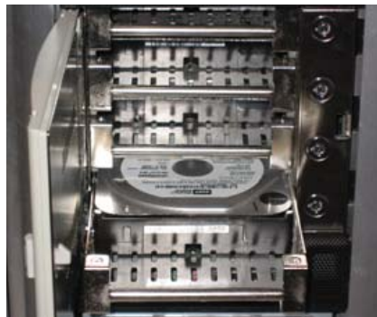
Figure 5. Pop open the RAID cage door, unlock the drives and pull them out for easy hot-swapping.
