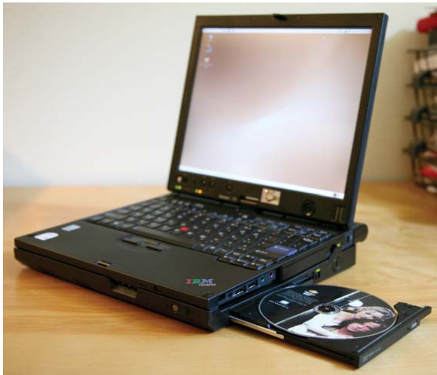
Figure 3. The included UltraBase docking station contains the DVD+-RW drive, as well as a multitude of additional ports.
