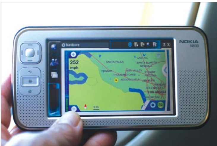
The Navicore, which stores its maps on a 2GB removable-SD card, was able to track progress along the ground during the flight from Santa Barbara to Los Angeles.
