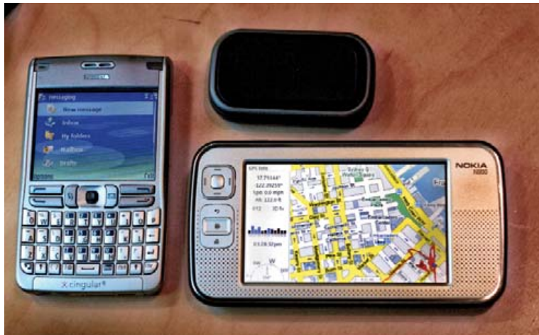
Three collaborating instruments provided by Nokia: the N800, an E62 phone and a GPS receiver. The phone used the Cingular/AT&T network.
