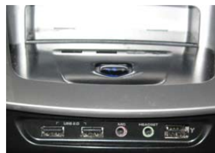
Figure 3. Under the lip below the power switch are duplicate USB ports, an IEEE 1394 port and audio ports.
