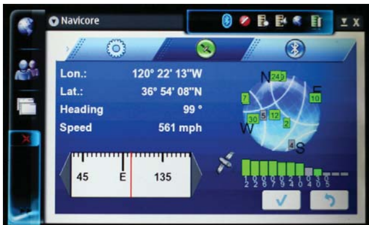
Here's the GPS data page in Navicore. The other two tabs on the top are settings (the gear) and Bluetooth.
