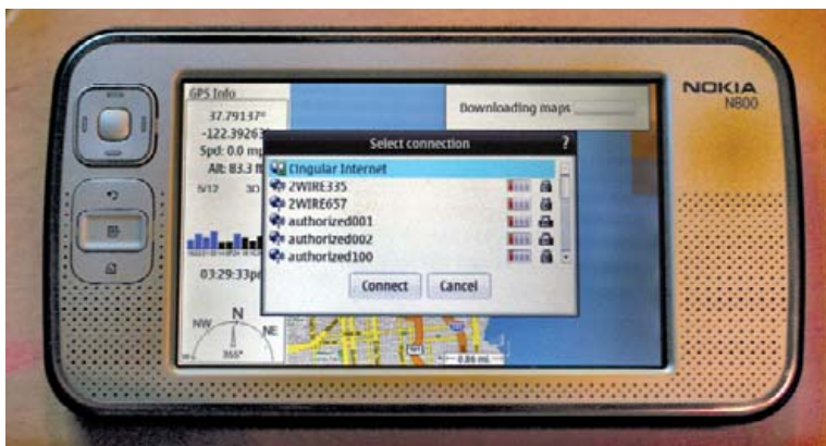
The N800 could see several Wi-Fi access points in addition to the cellular connection, and showed whether the connection was locked.
