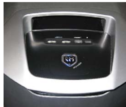
Figure 2. The power and reset switches along with USB ports and drive activity light are recessed into the top of the case.
