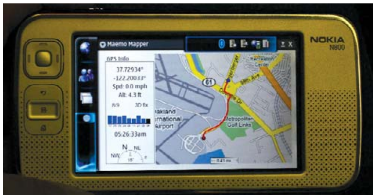
Maemo Mapper will create a track that leaves a red line. Here I'm taking a bus to a BART station from the airport in Oakland. The GPS receiver is in my pocket.
