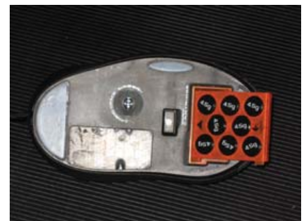
Figure 7. Add as many 4.5 gram weights to the puck as you like, and insert it into the mouse when you're done. This mouse is fully weighted.
