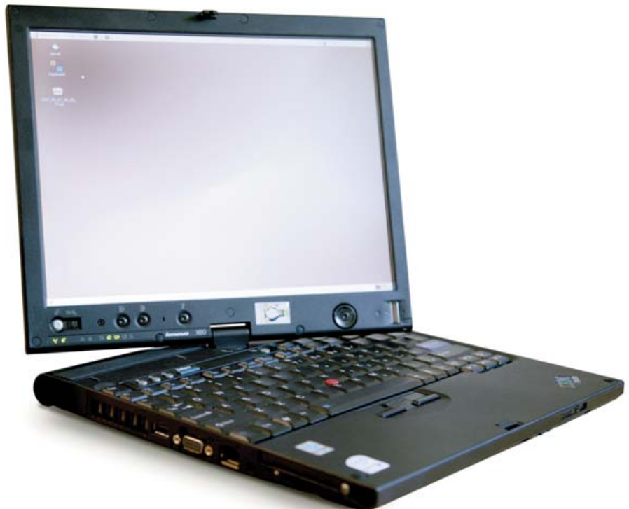
Figure 1. The Raven X60 has a 4,096dpi Wacom Tablet built in to the LCD display.
