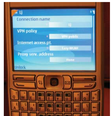
Figure 7. The final setup—give a name and Wi-Fi access point to the policy, and maybe set a proxy server too.
