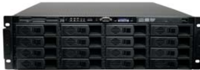
NAS 3008i 8TB Raw SATA Storage
