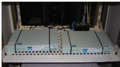
Figure 1. One set of route servers—IPv4 (Soekris 4801) on the left and IPv6 (Soekris 4501) on the right.
