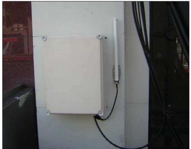
Figure 5. A CafeNet access point. The antenna is the small white rod on the right side of the box.
